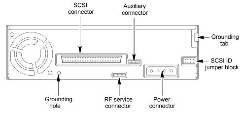
**Figure 2-1** Internal SCSI tape drive: back-panel components
